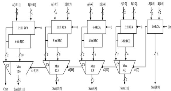
Figure 4: CSLA circuit using BEC Converter
